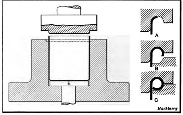
Fig. 13. Die for Curling Edges of Cylindrical Parts
